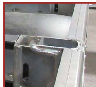
○ Welding to vertical I-beam cross members
